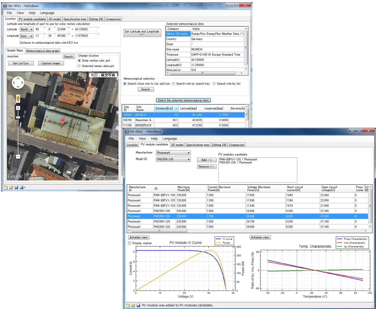
Generated results include not only system output power but power generated by PV strings and losses caused by devices such as inverters, cables, transformers and so on. These results are provided in both on-screen information and Excel-based reports.
